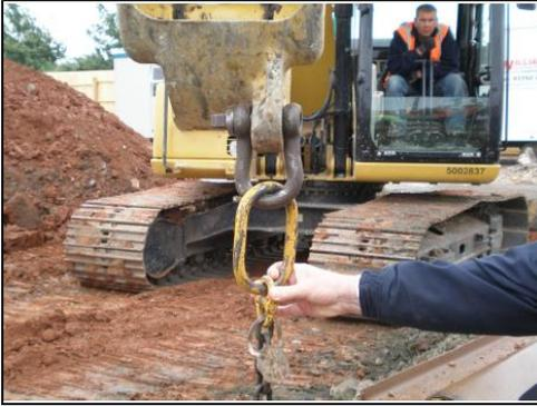
**Figure 11.** - Master link rotation restricted to approx.  $\pm 70^\circ$
