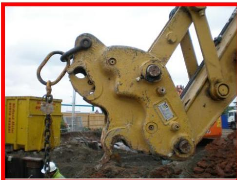
**Figure 14.** – Hitch tilted backwards with master link subject to bending
