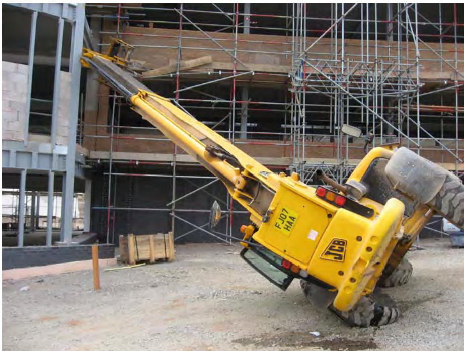
Figure 8 - Consequence of Instability
