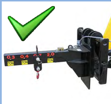
Carriage Mounted Lifting Point
