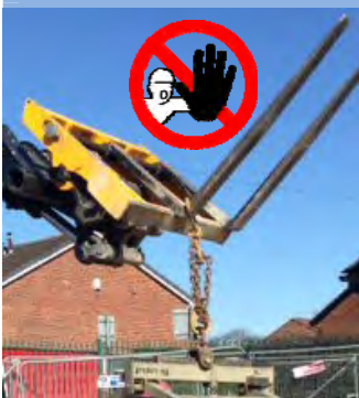
Sling Slipped over Fork
