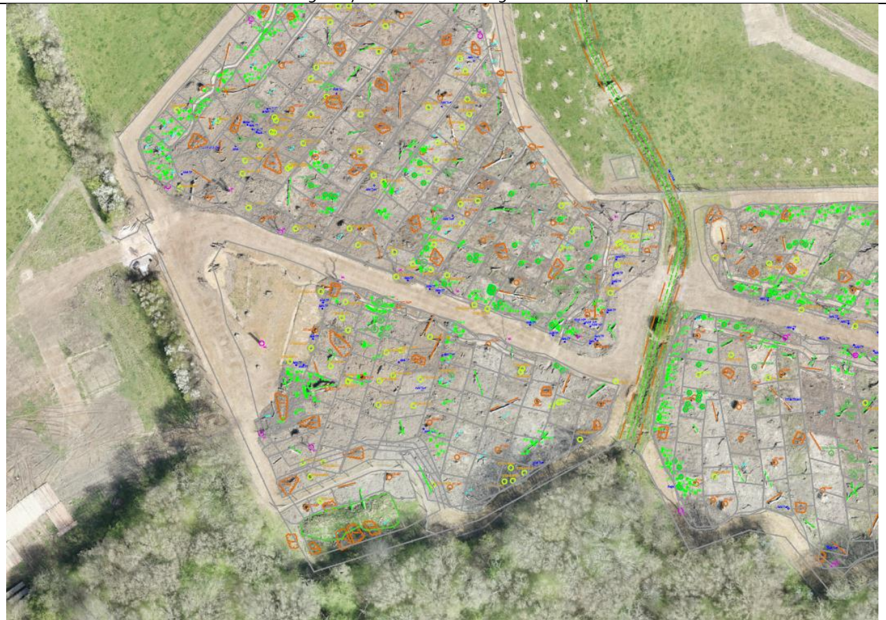
Above: The as built CAD drawing has been mapped onto a drone photo which will enable an aerial level of monitoring over time.
