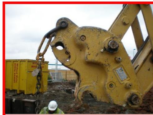
**Figure 15.** – Hitch tilted backwards with master link subject to twisting
