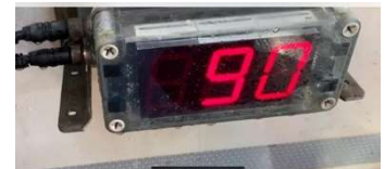
External VERIFI® display, indicating 90 mm slump
